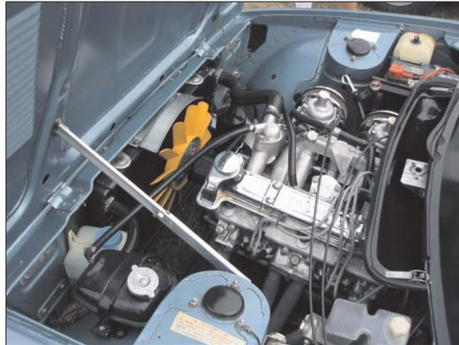
The engine bay of a typical TR7. The air cleaners are incorrect in this example and the valve cover should be medium blue.
